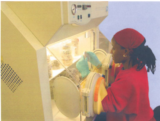
FIGURE 10 An anaerobic chamber. This rigid gas-tight cabinet is heated to 37°C and serves as an incubator as well as a place to work on the bacteria. It contains gloveless sleeves that seal around the operator's arms. This eliminates the dexterity problem associated with gloves that tend to be cumbersome. The gloveless cabinet requires that the air in the sleeves be evacuated before opening the entrance to the chamber. The airlock doors are open and visible in the picture. doi:10.1128/9781555818906.ch4.f10
